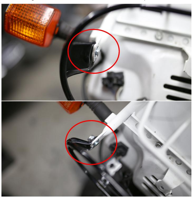
6. Install the new Chimera B2V Headlight into the headlight guard.
