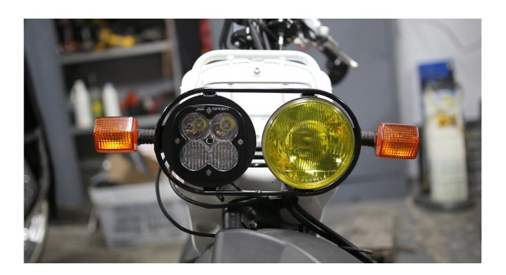
7. Wire the headlight to the existing headlight harness on the Ruckus. We recommend getting a H4 male headlight connector ETC-1104 or ETC-1105 (sold separately). You could also hardwire the headlight directly into the headlight harness, however it would require cutting the OEM headlight harness off.
