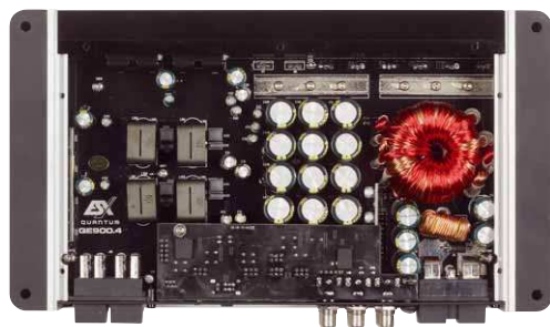
A lot in it, but not at all crammed: The ESX scores with a fat mains transformer and many small buffer capacitors. The class D coils are particularly strong
