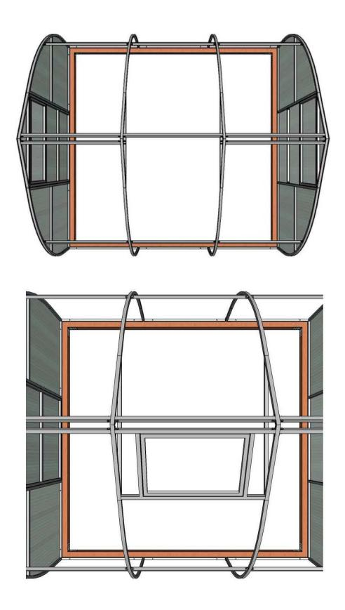
2. Attach the window frame to the vertical Studs #3 with the Countersunk screw 6x35mm #9 and Nut M6 #10.
