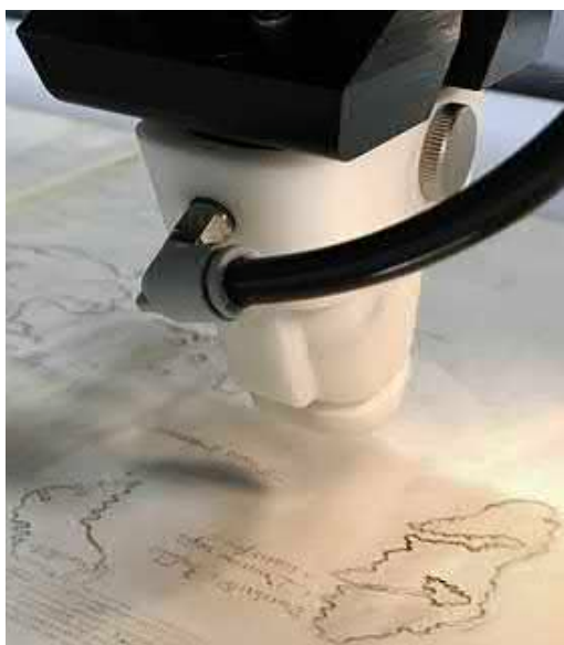
A scanning x-ray fluorescence spectrometer hovers over the map. The instrument created elemental maps revealing the distribution of elements throughout the map
