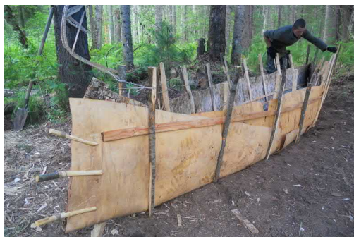
My first birch bark canoe construction in Siberia
