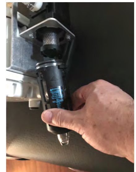
Put the black bulb back on pushing up and giving it a quarter turn to make sure it is securely connected.
