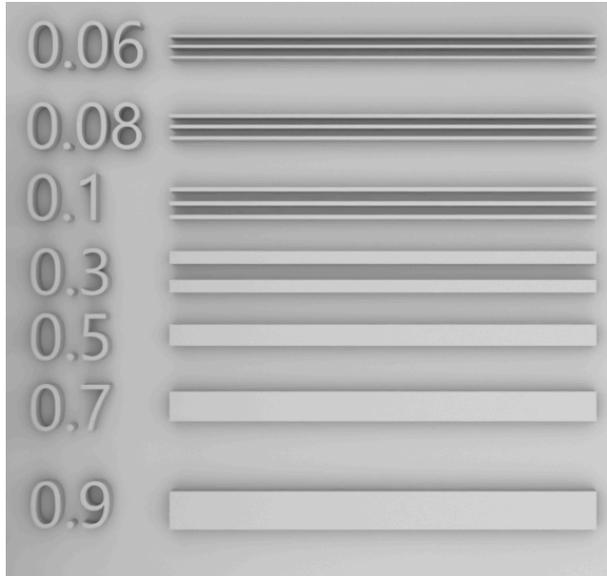
Minimum Engraved Detail Width, X-Y plane
