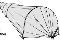
Standard rolls are 120 feet long to accommodate both 100-foot and 50-foot bed systems. A grower using a 50-foot-long bed system would cut the roll in half and still have five feet of extra material on each side of the bed to close the low tunnel's ends. Growers using a 100-foot bed system will likely want to trim the excess length.
