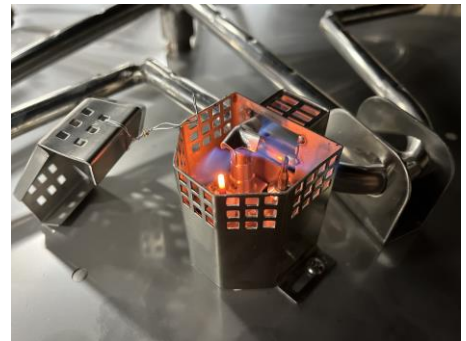
Figure 9.2 – Pilot flame coverage of thermocouple.
