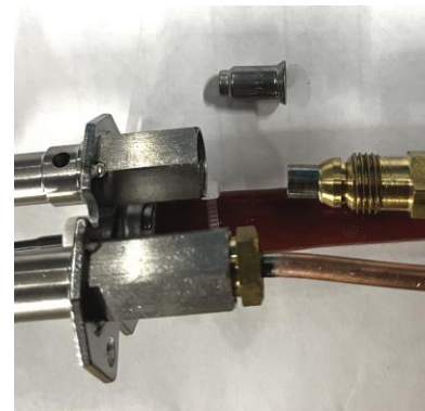
Figure 9.3 – Cleaning pilot orifice
