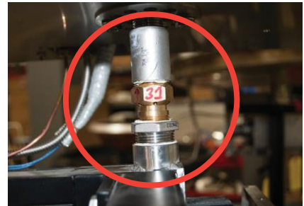
Figure 9.1 – Locating orifice for cleaning
