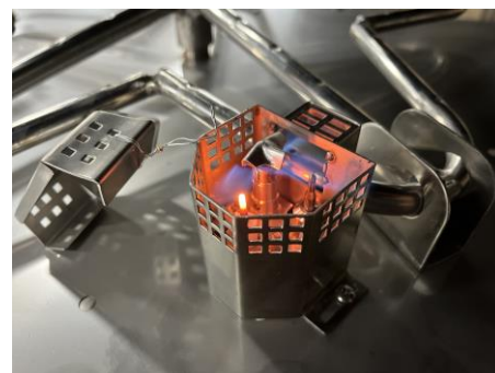
Figure 9.2 – Pilot flame coverage of thermocouple.
