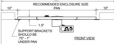
SPARK IGNITION BY AA BATTERY MATERIAL: 304 STAINLESS STEEL
