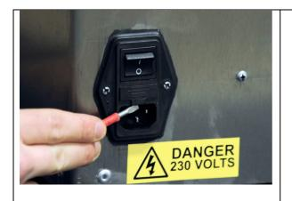
The iMelt system fuse is integrated within the IEC power socket.
