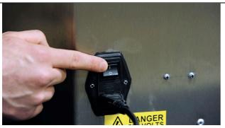
Step 3 – Turn the power switch to on (1)
