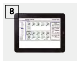
8 BMS integration. The cascade system can be easily integrated in a Modbus project thanks to the cascade manager.
