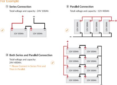
2. The following diagram is a reference on how to connect batteries in series and parallel using 12V100Ah-4S battery. Before connecting, each battery must be independtly fully charged. Please make sure that the voltage of each battery is within 0-0.3V after subtraction before connecting in series or parallel.
