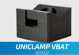
For use as either as hanger, using a 8mm threaded rod, or as a single fixing wall mount. The versatile Vbat can strap various sized piped ranging from 9-127mm in place with either a zip-tie or steel strap depending on application.
