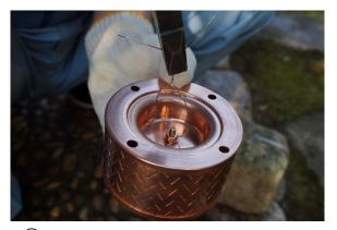
7 Make a loop with stainless steel wire on the back of the decorative weight while loosening the nut and wrap it around.
