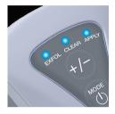
The LED lights cycle on and off from left to right while the unit is charging. All 3 LED's will turn on solid when charging is complete.
