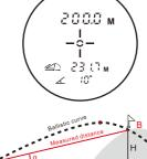
Long press ( to activate flagpole scanning mode, aiming at target B, \$\Phi\$ the flashing indicates the device is scanning when ( ) vibrating and ( ) is displayed in the upper left corner of the screen, the scanning measurement is completed, the distance from A to B. the Slope distance and the angle  $\alpha$  will be displayed on the screen accordingly.
