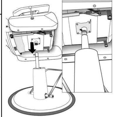
Step 3. Fix the pump by the fixing bolt of the pump.
