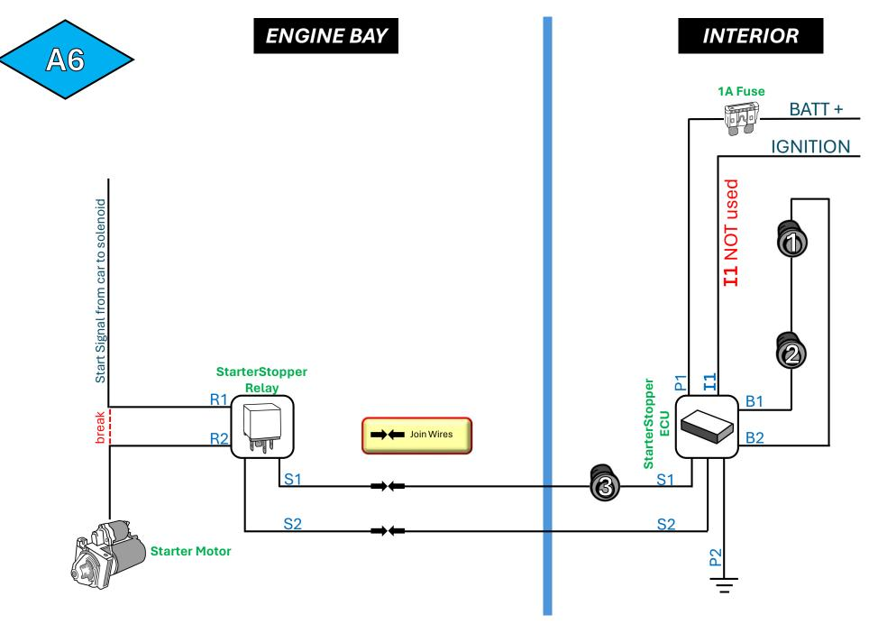
**Sequence:** Press TWO buttons (1 & 2) momentarily, then press and hold ONE button (3) whilst starting
