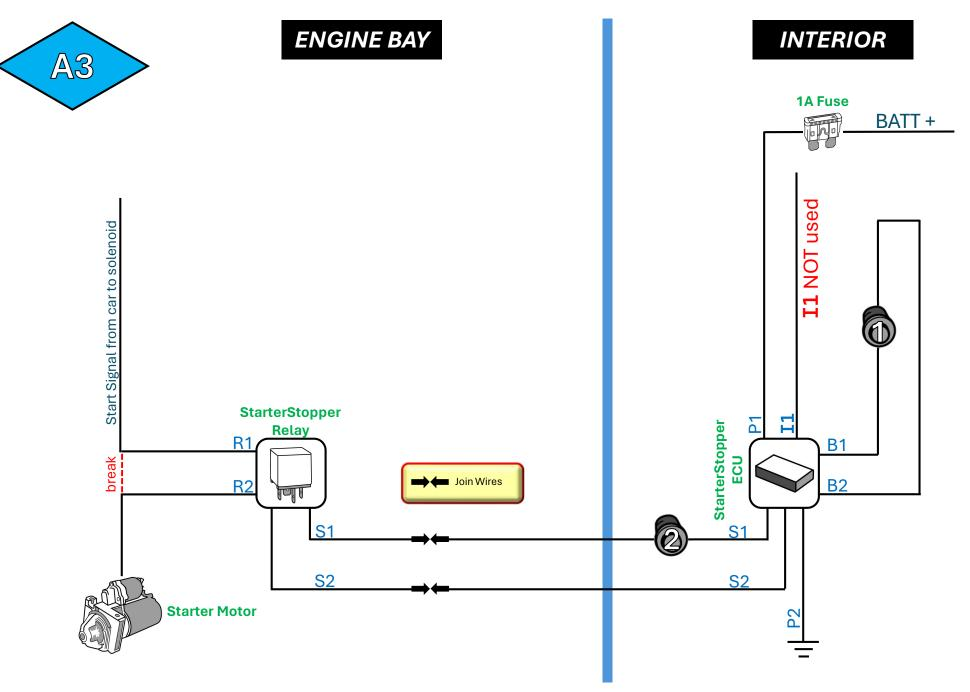
**Sequence:** Press ONE button (1) momentarily, then press and hold ONE button (2) whilst starting
