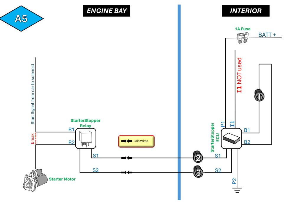
**Sequence:** Press ONE button (1) momentarily, then press and hold TWO buttons (2&3) whilst starting
