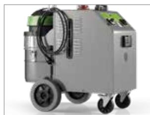
STRUTTURA IN ACCIAIO INOX, ASPIRATORE DI SERIE PER ASPIRARE LO SPORCO DISSOLTO, LIQUIDI E POLVERI
