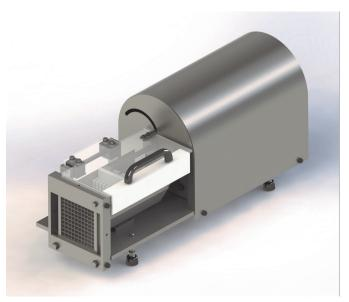
The product needs to be cut to the required length first, then loaded into the feed chamber of the baton cutter. On closing the lid the pneumatic ram is activated and a pusher block pushes the product through the cutting grid then retracts.
