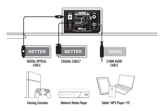
Note: Dolby Digital Plus, Dolby True HD, Dolby Atmos, DTS HD MA, DTS HD and DTS:X are not supported on Optical, Coaxial and Aux connections \* Cable not included
