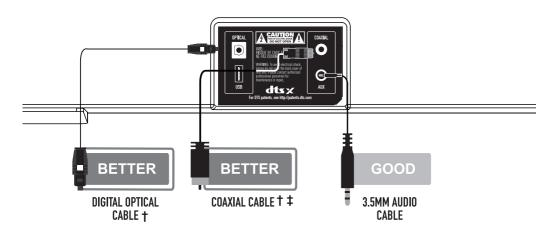
Note: Be sure to connect to a TV's audio output port, not an audio input port.
