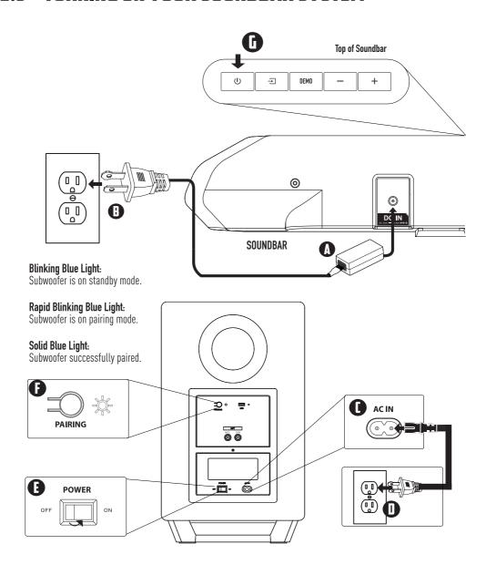
Tip: Once soundbar is powered off, the blue LED lights on the subwoofers will continue blinking for 10 minutes before going into standby mode. You do not need to turn off the subwoofers after each use.
