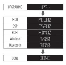
Note: If the soundbar is on the latest firmware, "FW UP TO DATE" will be displayed on the soundbar LED display.
