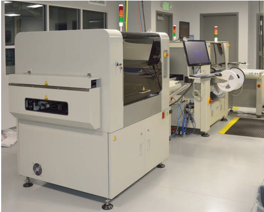
Campbell Company's fully automated SMT assembly line includes Manncorp's high-precision AP430 inline stencil printer, the 3-head MC-389 pick and place system, and a CR-5000 convection reflow oven. With a full complement of component feeders and connecting conveyors, the line bore a price tag of nearly $250K, yet Campbell management believes it paid for itself in 12-18 months.
