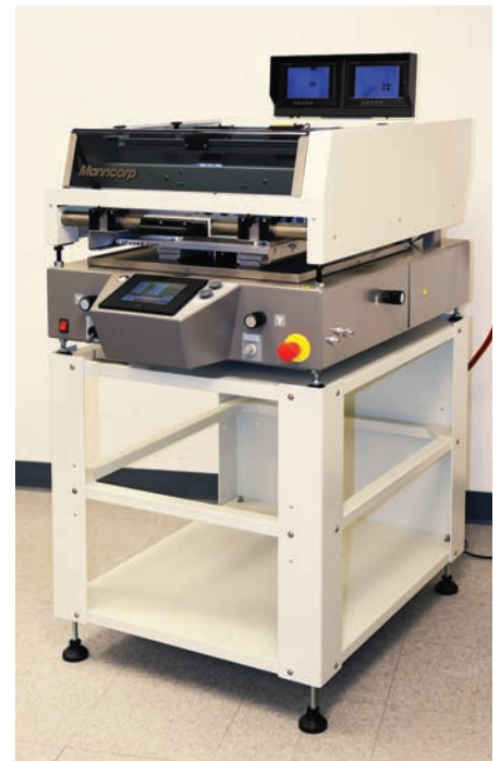
For increased printing accuracy and easier stencil to board alignment, Sensorcon chose Manncorp’s PB2300 vision-assisted semi-automatic stencil printer. Like their original pick and place machine, their manual stencil printer will now be dedicated to prototyping and new product development.
