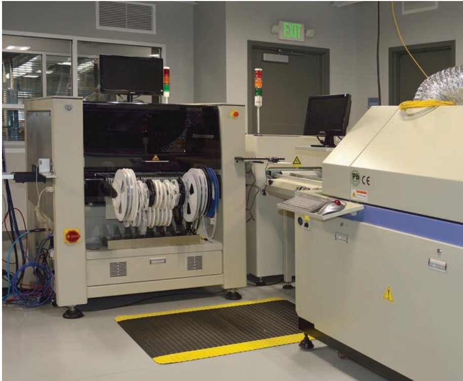
Due to space limitations, a 90° turning conveyor is positioned between Campbell Company's 3-head MC-389 pick and place machine and their 5-zone CR5000 convection reflow oven. Single-sourcing a complete turnkey SMT production line from Manncorp provides such benefits as seamless equipment integration, special package pricing, coordinated delivery, installation and training, and extended warranties.
