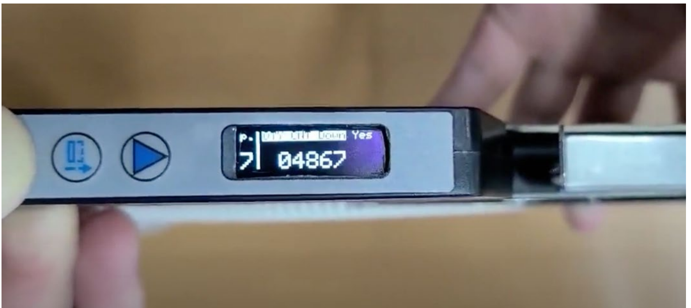
Figure 1: View component quantities, feeder slot locations, part numbers and values, and more on the built-in display.
