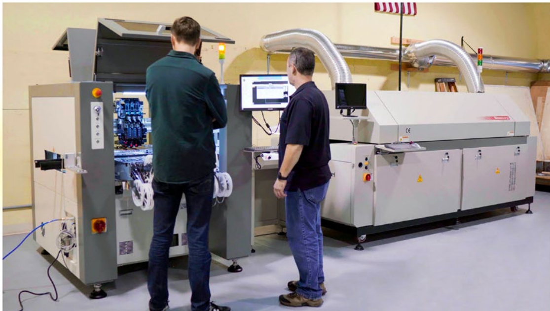
Figure 2: The Critter & Guitari high-mix production setup with a 160-feeder port pick-and-place machine.
