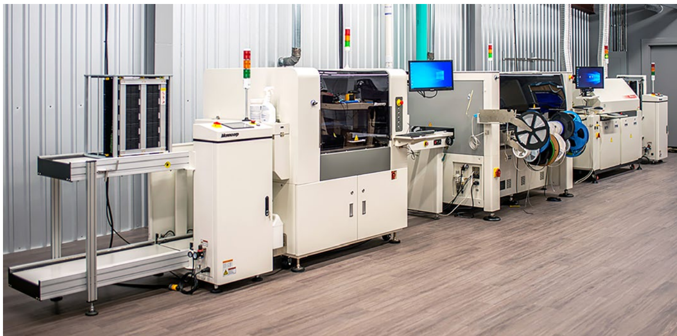
Figure 4: A full SMT equipment line installed at CoralVue as supplied by Manncorp.
