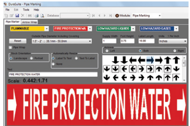
Pipe marker designed with a single line of text
