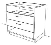
Note that there are two (2) front corner Levelers located behind toe kick and accessible through drilled access holes in cabinet floor. Remove plastic plugs from access holes in order to perform leveling adjustments in next step.
