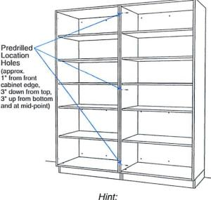
Use clamps to hold cabinets together during this process.
