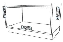
NOTE: Turn clockwise to lift, counterclockwise to lower.
