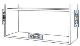
Securely attach cabinet to building structure through both Mounting Rails, in the locations illlustrated in Step #2.
