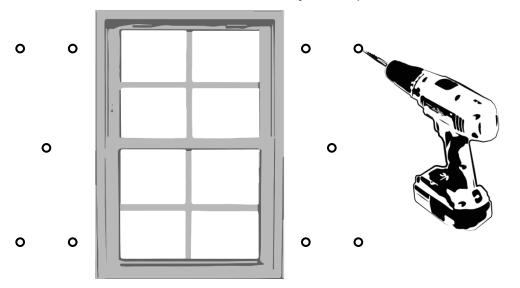
6. Use a hammer to lightly tap all 10 wall anchors into holes until flush with the surface of the wall.
