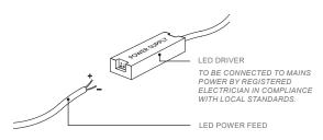
1. Connect LED power feed to LED driver.
