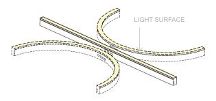
Avoid bending LED Neon within the first unit (units are clearly marked with dashed lines on the sides of the product)
