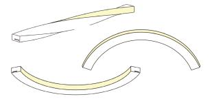
LED Neon can be bent up to the defined "minimum bend radius" (60mm for Neon Edge)
