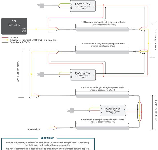
to prevent resulting overloading and overheating if one power supply fails.
