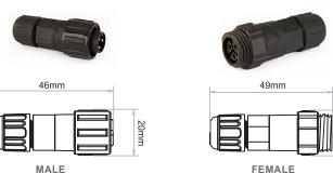
CONNECTOR TOLERANCE +/-2MM
