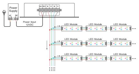
6.2 If one controller is not enough, can add extra power repeater to expand the power output.
