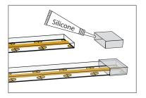
Please note drawings are an installation guide only. Each LED Ribbon Strip application may have variable factors. Cable size may need to be specified to limit the voltage drop throughout the circuit.
