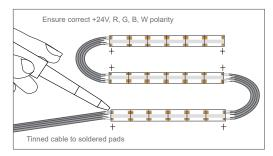
Please note drawings are an installation guide only. Each LED Ribbon Strip application may have variable factors. Cable size may need to be specified to limit the voltage drop throughout the circuit.
