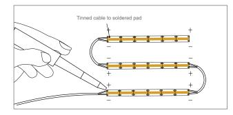
Please note drawings are an installation guide only. Each LED Ribbon Strip application may have variable factors. Cable size may need to be specified to limit the voltage drop throughout the circuit.
