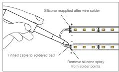
Please note drawings are an installation guide only. Each LED Ribbon Strip application may have variable factors. Cable size may need to be specified to limit the voltage drop throughout the circuit.
