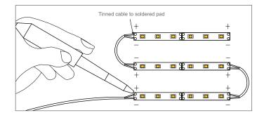
Please note drawings are an installation guide only. Each LED Ribbon Strip application may have variable factors. Cable size may need to be specified to limit the voltage drop throughout the circuit.
