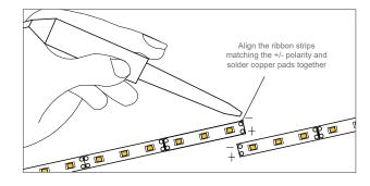
Cut and trim the cable to the appropriate length. Solder the wires onto the end of the ribbon strip ensuring the correct +/- polarity.
