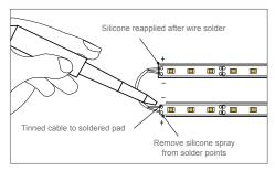
Please note drawings are an installation guide only. Each LED Ribbon Strip application may have variable factors. Cable size may need to be specified to limit the voltage drop throughout the circuit.
