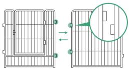
Align the circular rings on the gate panel and the mesh panel. Please note that the height of the rings is different.
