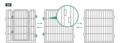
Align the circular rings on the gate panel and the regular panel. Please note that the height of the rings is different.
