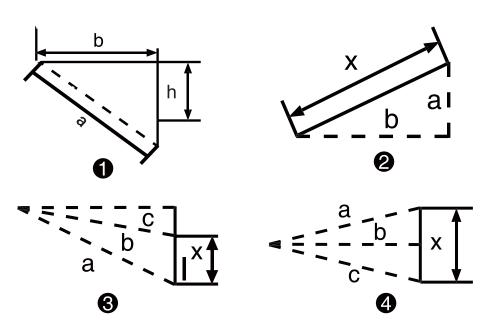
There are four preset modes for the instrument to measure the distance of one side of a triangle by using the Pythagorean theorem.
