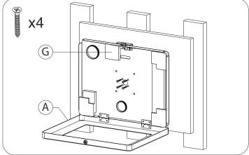
2A. Align innermost VESA holes to the drilled holes and screw in the (4) screws (G) until securely tightened.
