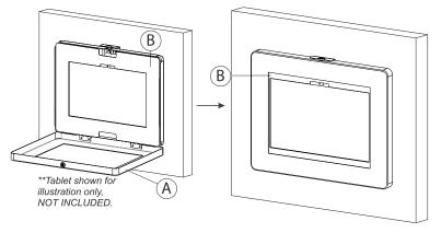
5A. Lay-in correct masking insert from bundle (B) as needed the correct fitted look for your device.
