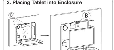
3A. Find the appropriate size foam padding (B) for the tablet you wish to use. Make sure device is compatible for the enclosure. If having power/data cord attached to tablet, slide it through the back of the foam as shown and out the opening in the back.
