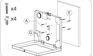
1A. Insert the (4) wall plugs (E) to the wall drilled holes. Then, align outermost VESA holes to the drilled holes and screw in the (4) screws (G) until securely tightened.
