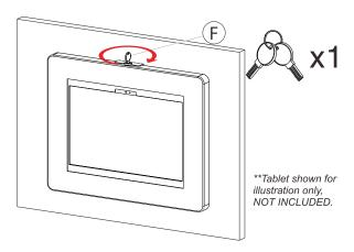
7B. Insert the key (F) in the keyhole on top of the enclosure, and turn clockwise to lock the enclosure in place.
