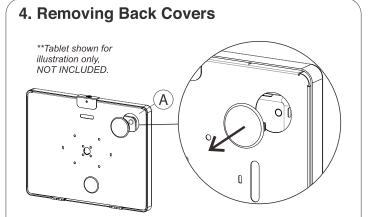
4A. When installing device into the enclosure, identify where the camera is. Then simply remove and pop out the cover prior to mounting or setting up tablet to properly expose camera.
