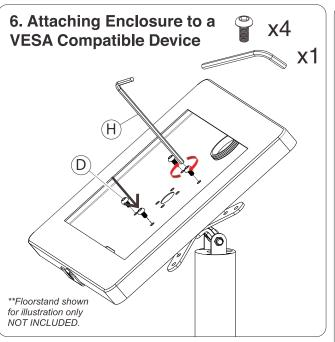
6A. Align enclosure holes to VESA plate holes. Screw in the screws (D) above using provide allen key (H).
