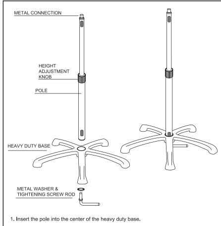
2. Place metal washer over tightening screw rod, then screw into the bottom side of the stand base center, turning clockwise to tighten.
