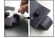
Place the screw bolt from each wheel through the metal base, then place a nut cover over the top of each. Screw down clockwise by hand, then use wrench to tighten
