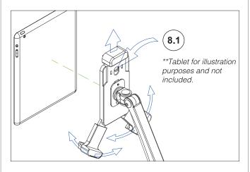
8A. Press the switch (8.1) to allow the top holder arm to adjust as needed. You should stretch it to max distance. Then place your device in and first make sure the two bottom corners of device are in the bottom two holder arms and securely setup as shown in step 7. Then push the top holder arm and retract back to the top edge of the device for a comfortable and secure fit.
