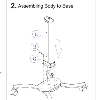
2A. Take the now assembled base with wheels, and align holes of
