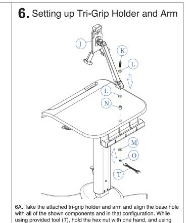
screwdriver (not provided) rotate in screw (K) until securely fastened.
