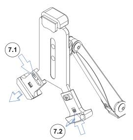
7A. Identify the switches on the holder (7.1 and 7.2). Pressing switch 7.1 allows you to extend the holder arms to match the device size bottom corners. Pressing switch 7.2 allows you to adjust to the thickness of the device. Make sure to retract for any space so it's a secure and tight fit.
