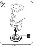
Lock part C to the assembled component.
