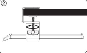
Turn the knobs on the C-clamps to secure the keyboard tray to your desk.
