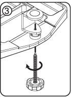
Insert screw into the C-clamp
