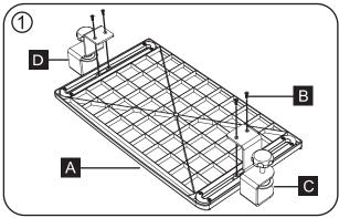
Attach the 2 C-clamps using the screws provided.
