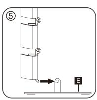
Attach part E to the bottom of the chain.
